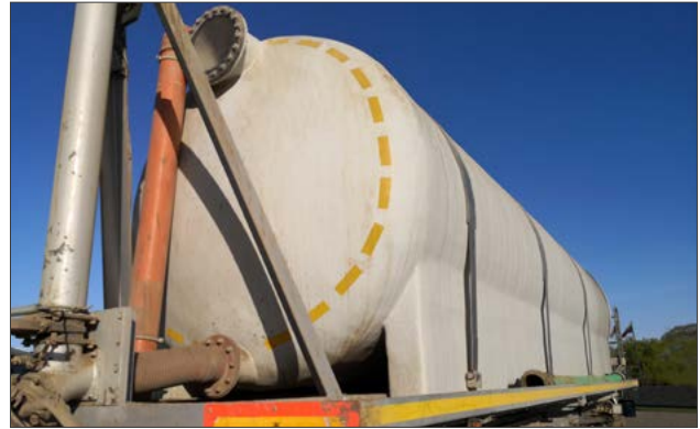
Transport Tanks can be mounted on trailers or in open steel containers.
