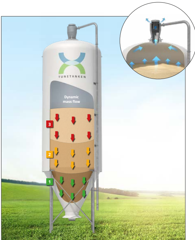
An efficient blow-in system with a cyclon and ventilation distributes the media, ensuring that it doesn't get packed too tight, and minimises risk of condensation.
