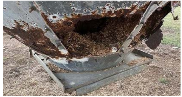
Fiberglass silos do not corrode! Salt and ammonium in the feed, combined with water condensation, result in corrosion, which composite materials are resistant to.
